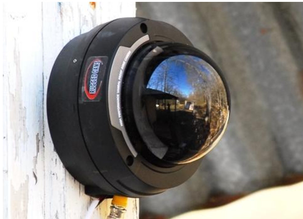
Figure 11: Rugged Cams Sentry 700 HD Infrared dome camera. Photograph: Chris Buntenbah.
