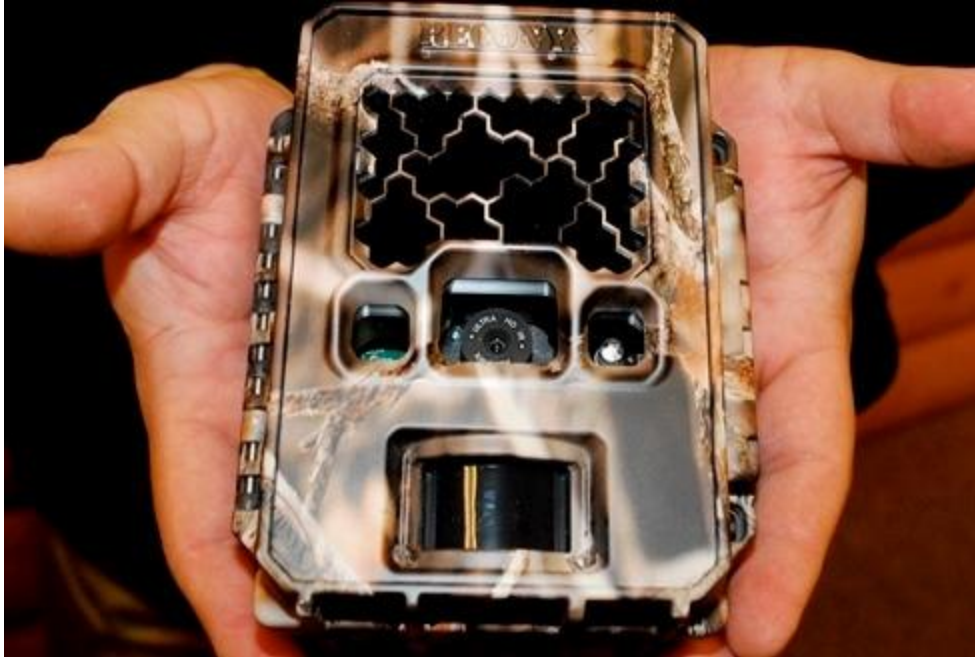
Figure 7: Reconyx HC600 Hyperfire, with “covert” infrared. Photograph: Chris Buntambah.
