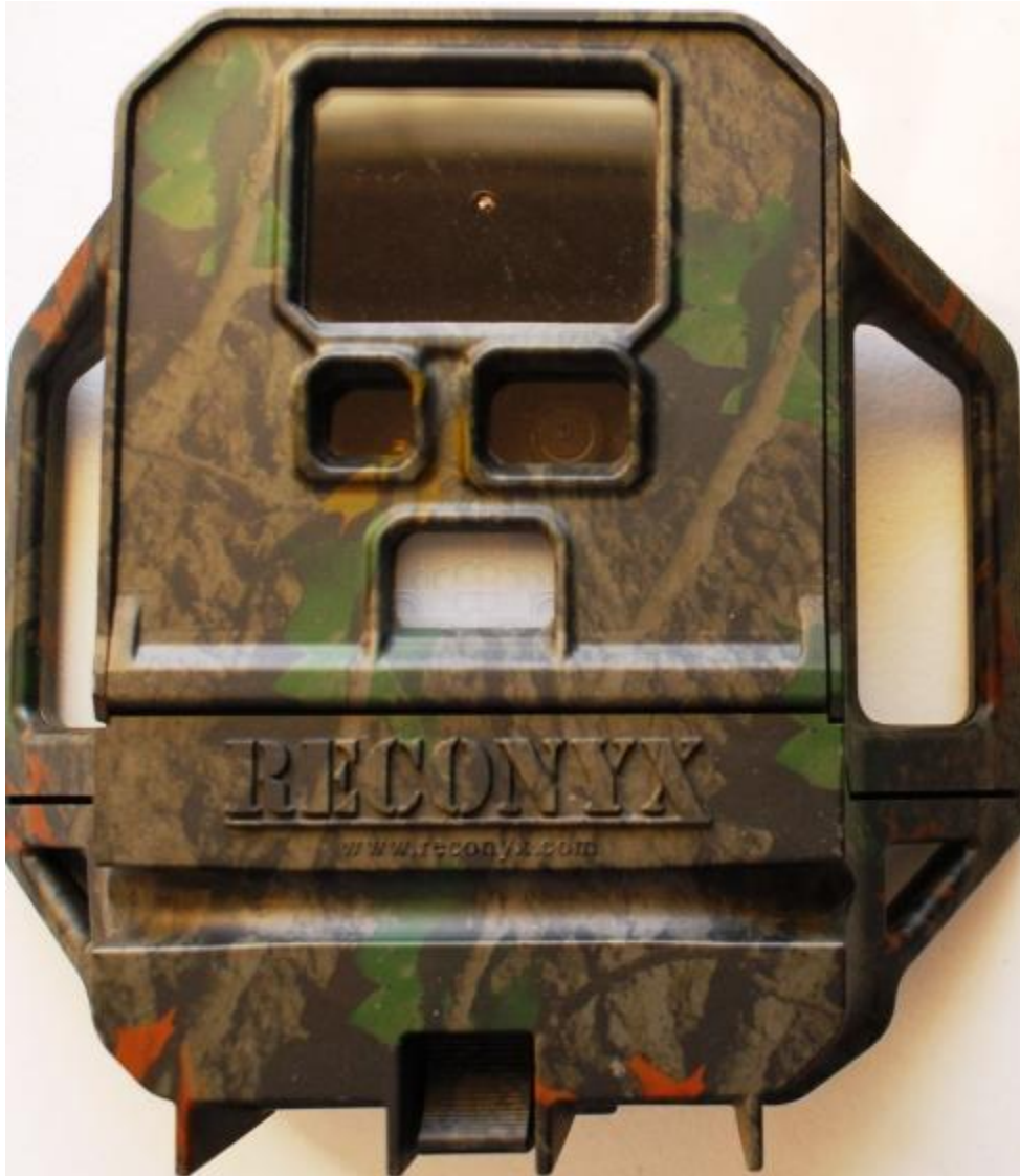
Figure 9: Reconyx RC60 Covert game camera. When the infrared lights trigger, there is no "red glow," thus supposedly making the camera's "covert" illumination undetectable. Photograph: Chris Buntambah.
