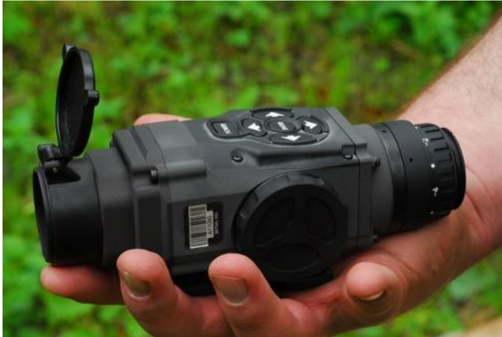
Figure 3: The ATN ThOR 320 60hz thermal optic. The NAWAC procured two of these thermal optic devices. Photograph: Chris Buntambah.
