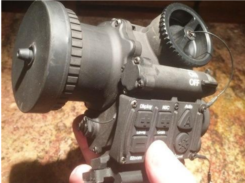
Figure 5: FLIR Thermosight T-50 thermal scope. Photograph: Paul Bowman, Jr.
